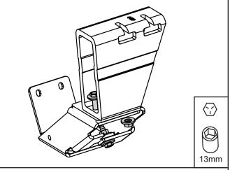
Assemble Linkage to bracket assembly using a 15mm Socket or wrench. Use supplied flange Bolts (#9). Torque Bolts to 20ft-lbs.
