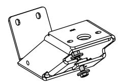
Using a 13mm Socket and wrench assemble the frame mount to the lateral mounting brackets. Use bolts (#10) and nuts (#13). Note orientation of brackets. Torque bolts to 16 ft-lbs.
