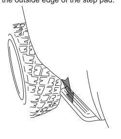
To retract, gently kick up on the underside of the step pad.
