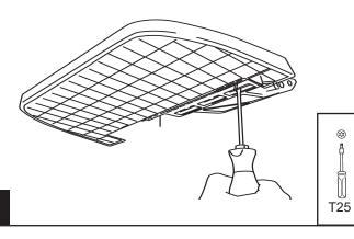
Verify step pad alignment to body line of vehicle.
