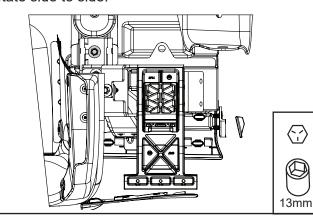
Using supplied M8 hardware Bolts (#12) Nuts (#13) mount support bracket to inner bed panel and lateral bracket as shown.
