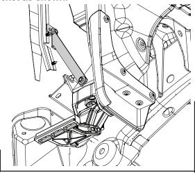
Using supplied M8 hardware Bolts(#12) Nuts (#13) and M10 bolt (#9) and nut (#8) mount frame support bracket to lateral bracket as shown.
