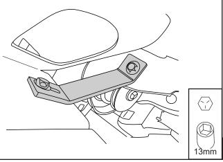
Locate factory bed bolt. Using a 13mm socket or wrench remove bolt.
