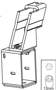
Assemble Linkage to bracket assembly using a 15mm Socket or wrench. Use supplied flange Bolts (9). Do not tighten bolts, leave loose to adjust linkage in a later step.
