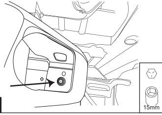
Set linkage assembly into position and tighten bed bolt. Torque bed bolt to 40ft-lbs.
