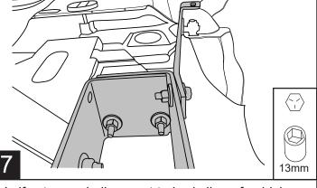
Install step pad (#2) onto linkage. Torque to 5ft-lbs. 6.5' bed applications center step pad on linkage (As shown).
