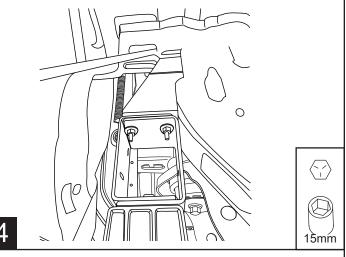
Assemble Rear support Bracket (#5). Use Bolt (#12) and nut (#13) on linkage assembly and Bolt (#12) and threaded nut plate (#8) on Frame. Torque bolts to 16ft-lbs.
