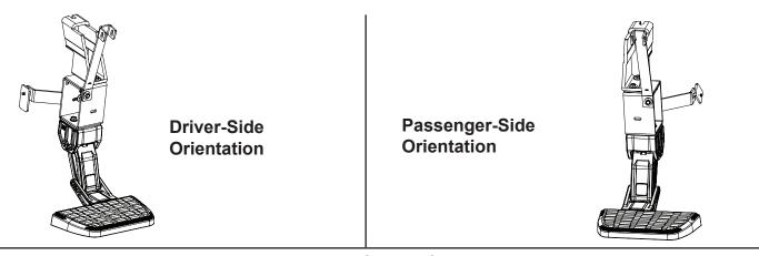
For 6.5' bed lenghts components must be configured for Passenger or Driver-side as shown.
