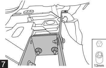
Verify step pad alignment to body line of vehicle.
