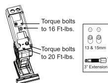
**B.** Install bracket to linkage, using supplied bolts (12). Hand tighten bolts then torque from steps A & B. See above for torque spec.
