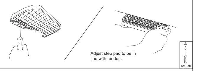
Verify that step pad (2) is parallel to the bottom of the body line. A shim (14) is provided to level out step pad. See image for explanation.
