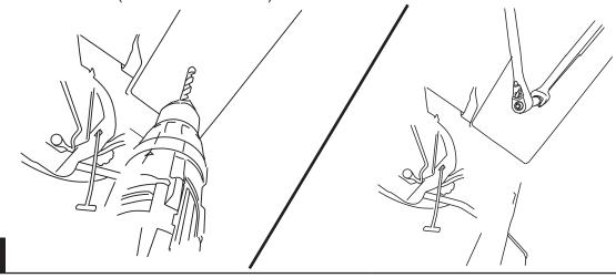
Reassemble Bedstep Assembly under truck and snug the three locations up.
