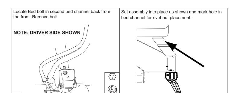
Once hole is marked remove Bedstep Assembly and pre drill using an 1/8" drill bit. Drill to 17/32". With Rivet Nut Tool held in place with 9/16" wrench, tighten Hex Bolt until Rivet Nut deforms and secures itself to the sheet metal (20 ft-Lbs. or 4 turns). Remove Hex Bolt and Rivet Nut Tool.
