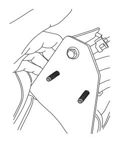
Set frame mount into position and tighten two bolts.
