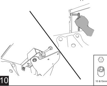
Using "Bracket E" and provided flange head bolt re attach brake cable bracket. Do not tighten.
