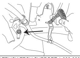
Bolt Bracket A up to bed support rib.
