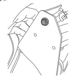
Install Bracket G onto Bracket F and use provided bolts, washer and nut to attach bracket to Front support rib.
