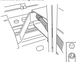
Using a 13mm Socket tighten 2 bolts holding Frame mount to bed channel. Do not tighten bolts
