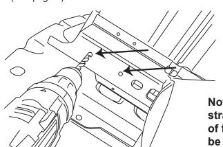
Note: On passenger side Ground strap may interfere with mounting of frame mount. Relocation may be required
