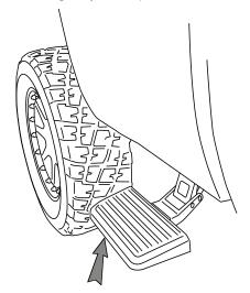
Note: If linkage or step pad comes in contact with the body use provided washer. Remove white bumper between linkage arms and insert washer and replace bumper.
