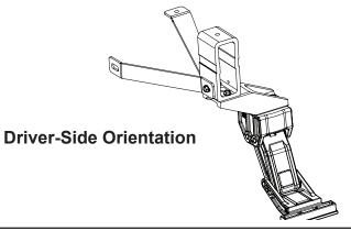
Using a 15mm Socket assemble Lateral mount onto Linkage assembly. Torque bolts to 20 ft-lbs. Note: Drivers side shown. Mirror for passenger side(See image in step 1 for passenger orientation).
