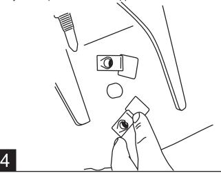
Offset the step pad forward and secure using provided PT Screws. Tighten to 5 ft-lbs using T25 torx bit. Note: Driver side shown
