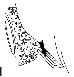
Set linkage in place and tighten bolts using a 15mm socket. Torque bolts to 20 ft-lbs. Note: Image shows Crew Cab short bed. Bed mount may not be present in other applications.
