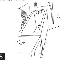
Adjust step pad to be in line with fender and torque bolts from Step 2 to 20ft-lbs.
