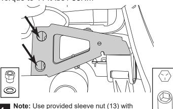
**Note:** Use provided sleeve nut (13) with washers (14) when short studs are present.
