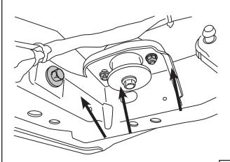
Using a 15mm wrench assemble steel bracket to Linkage assembly. Torque bolts to 20 ft-lbs.
