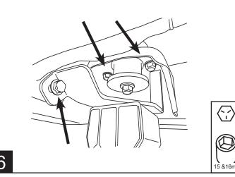
Offset the step pad towards the left and secure using provided PT Screws. Tighten to 5 ft-lbs using T25 torx bit.
