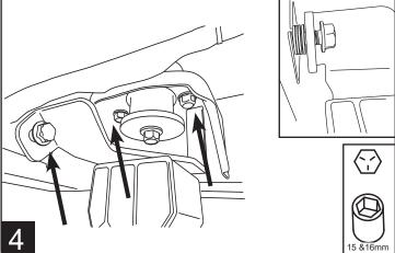
Thread M8 bolt into threaded bracket from step 3. Torque to 16ft-lbs.
