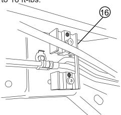
Pre thread upper M10 flange head bolt onto frame mount. Slide linkage into position and thread in lower flange head bolt. Motor faces front of vehicle.
