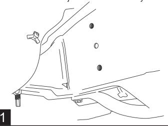
Using provided flat head cap screws attach frame mount extrusion to front set of threaded holes. Torque screws to 16 ft-lbs.
