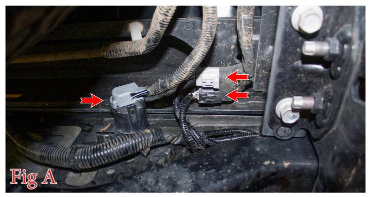
2. Remove the trailer plug by pressing in the two tabs on the back side of the plug and pushing the plug out the front side of the bumper. (Fig B)
