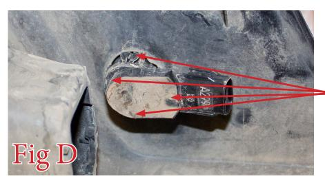
Press in all the tabs on the back side of the parking sensor to release it from the bumper.
