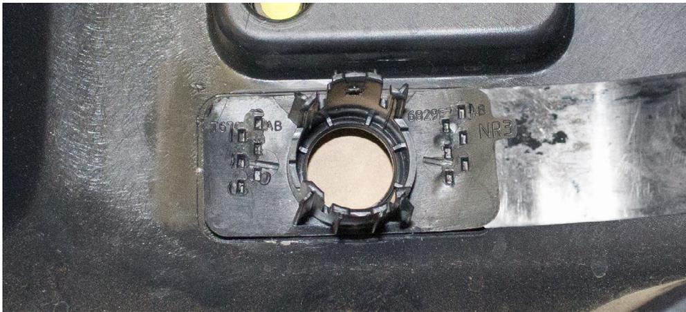
**Use a scraper to separate the mounting plate from the bumper**
