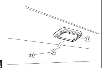
Using supplied butt connectors, connect the lamp wires. Red to Red, Black to Black. Heat the shrink tubing on the connecters to seal wires.
