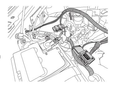
Route shorter leg of harness down Passenger-side wheel well and longer leg of harness down along driver side wheel well. Attach wire harness with supplied 7" cable ties (15).
