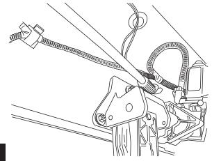
Remove driver side front kick panel and door sill plate. Roll back carpet to access hole for passing trigger wires into cab of vehicle.
