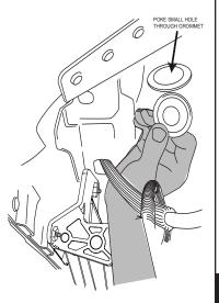
On Super Cab models, use a 9/32" drill bit to drill hole through floor and insert grommet (#8) that is supplied with kit. Thread the wires through and apply silicone sealant.
