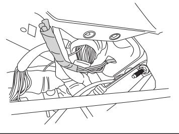
OBD II Connector located below driver side steering column.
