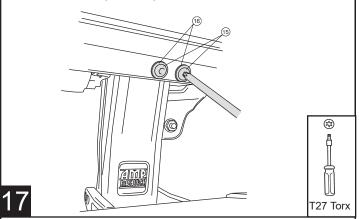
Using a T27 Torx driver torque bolts to 6 ft-lbs.
