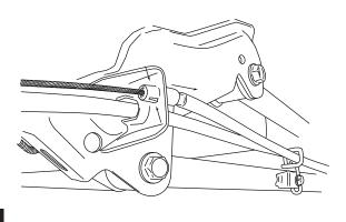
After gaining enough slack, detach brake cable as shown below. This detachment point is located just to the rear of the adjustment nut.
