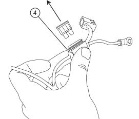
Connect power leads from Controller, Red to positive battery terminal and Black to the vehicle body ground as shown.
