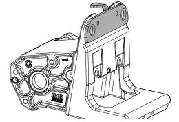
Using a 13mm wrench tighten two hex bolts on linkage. Torgue to 16 ft-lbs. Torgue bolts from step 15 if present to 50 flt-lbs.
