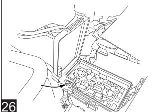
Locate the vehicle's Door Ajar Switch wires on the removed connector as indicated in chart and diagram below according to vehicle model year.
