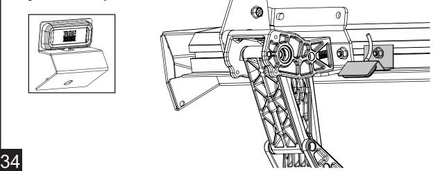
Using supplied butt connectors (27), connect the lamp wires. Red to Red, Black to Black. Once Crimped use heat gun to shrink tube. Close and wrap conduit with electrical tape. Secure all loose wires with cable ties. Pull lamp wires upward to avoid any wire snagging.
