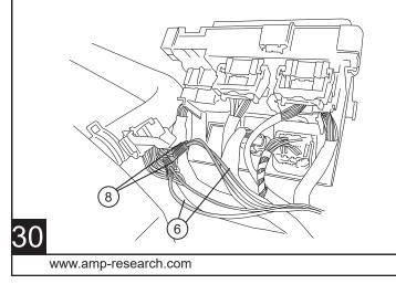
Locate and remove Black Connector with Gray latch on bottom side of fuse box (labeled "G" where connected to fuse box).
