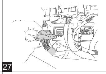
Splice Power Step trigger wires into the Door Ajar wires with provided Posi-Tap<sup>™</sup> splicers. The Power Step trigger wires color coordinate with the factory Door Ajar wires. Follow the steps below to correctly splice wires.
