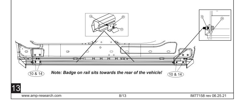
Thread supplied bolts 2x (9) into Front Drive Linkage. Repeat step for Rear Idler Linkage. Do not tighten.
