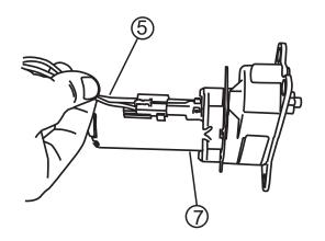
Slide rubber grommet on wire harness into slot of motor cover. Install motor cover onto motor.
