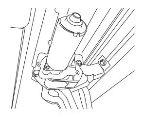
Affix LED lamp (#20) to Light bracket (#21) on rail. Slide bracket into desired position and tighten using 5/32" Allen key.
