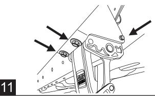
Attach motor to linkage. Using a 13mm wrench Torque to 36 in-lbs.
