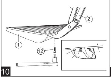
Using a 13 mm socket torque linkage bolts to 16ft-lbs. Next use a 10mm socket torque linkage spacer bolt (#19) to 8 ft-lbs. Once linkages are tight cycle board to verify steps deploy under own weight and clear rail endcaps.
