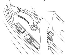
Connect harness to motor. Secure harness with tie wraps.
