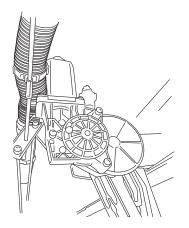
Using the two 11" zip ties (20), mount controller (6) to support arm next to battery. Plug in harness (Ensure that locking tabs engage)
