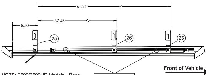
**NOTE:** 2500/3500HD Models - Rear mount on passenger side of vehicle will need to be moved forward from last mounting hole to second to last hole. Approx 15-1/4".
