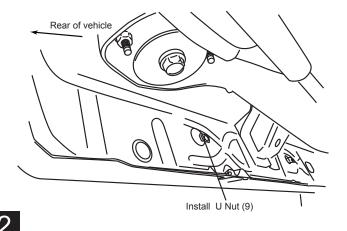
Set rail up into position. Starting with the rear bracket work towards the two front brackets. Attach Bolts 2x (8) and Nut 1x (9). Snug to body do not tighten! Note: Forward and middle bracket may not need nut if threaded
