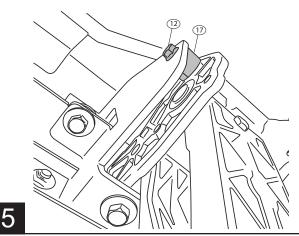
Slide mounting T-nut into position, Center board in rail pocket. Tighten fasteners (14) to 10 ft-lbs.
