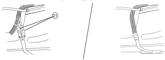
**OBD II install:** Use Supplied Posi-Lock<sup>™</sup> (7) connectors to attach the Plug and Play Module (24) to the Harness. Attach matching colors on the harness to the wires on the module. Plug in module (24) to OBD II port on the vehicle. Secure harness with supplied tie wraps.
