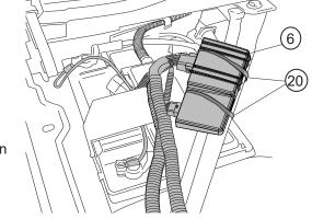
Remove power fuse. Attach power lead (RED wire) to positive pole
