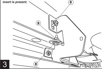
Thread supplied bolts 2x (8) into Rear Drive Linkage. Repeat step for Front Idler Linkage. Do not tighten.
