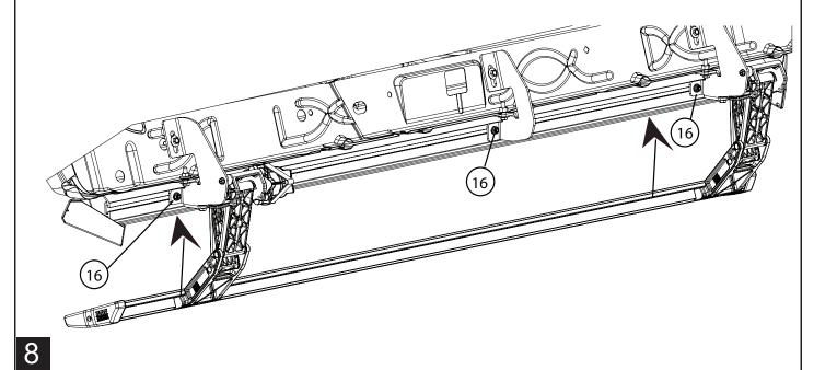
**A**: Using a 13mm socket tighten 3 bolts along pinch weld first. Torque to 16ft-lbs.
