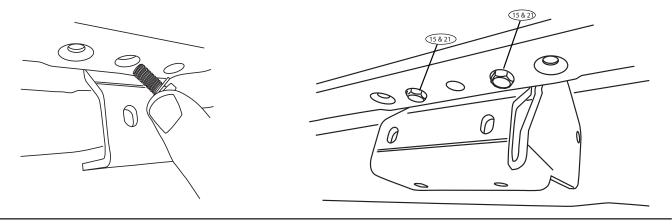
Insert 7 Carriage Bolts (17) into slot on Rail (4). Insert from either end of rail. Add 2 Light Brackets (25) on the 3rd and 5th bolt. Insert Flange Nut (18) onto bracket tab to attach light brackets into position shown. Leave loose to allow for adjustment.
