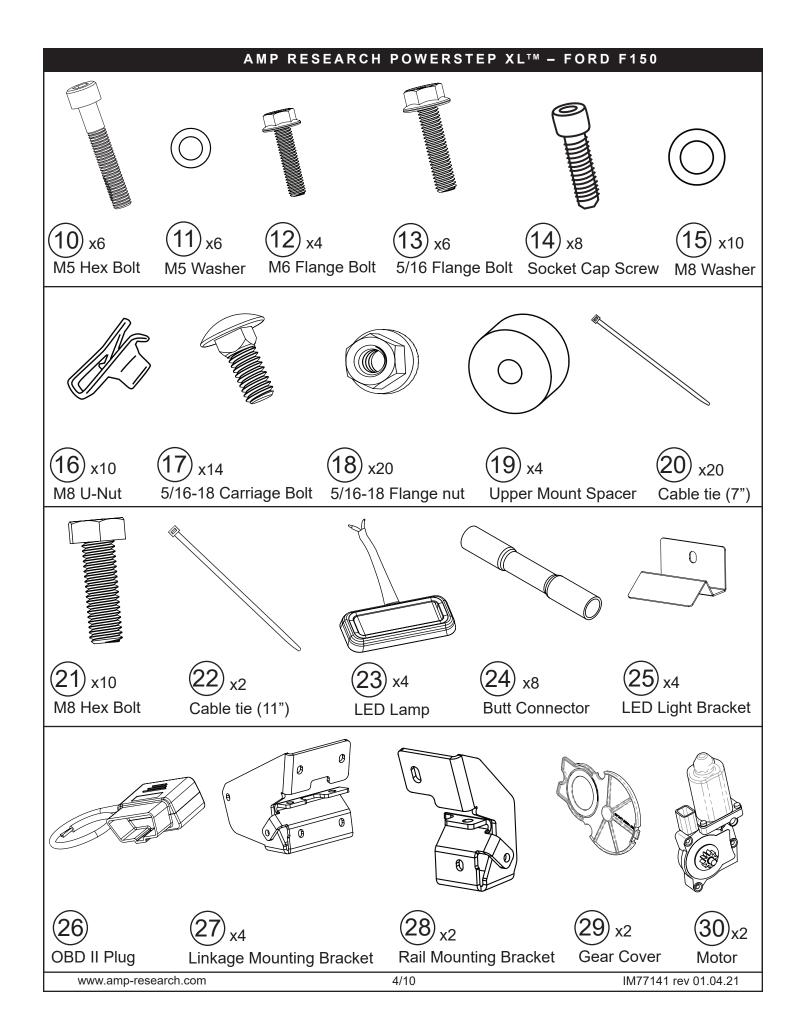
Locate mounting points. First middle and last set of holes on the inner sill. Install 5 U-Nuts (16) in
