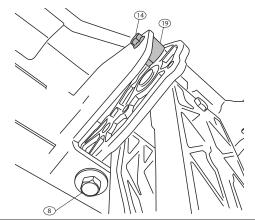
Attach motor to harness. Using a 4mm hex Torque to 36 in-Lbs.
