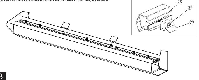
Using provided captive washer M8 bolts (8) install upper bracket hardware to brackets. Do not tighten.
