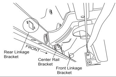
Set Brackets into position and use provided M8 Bolts (21) and washer (15) on outside and provided M8 nuts on the backside. Do not tighten.
