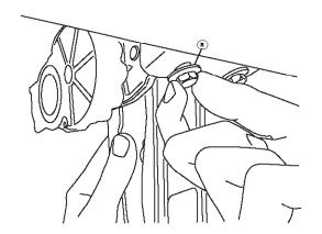
Install provided spacer (19) and M6 bolt (12) into upper mount as shown on both the Drive and Idler linkages. Do not tighten.
