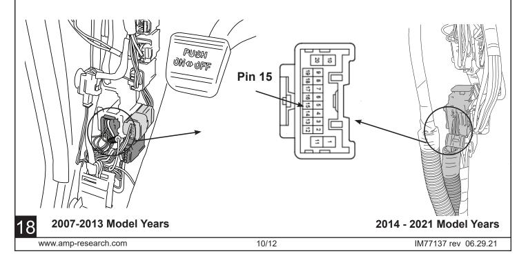
Locate the 22 pin connector at the bottom of the passenger side kick panel area. See pin connector locations for corresponding model years.
