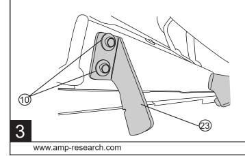
Repeat Bracket installation on passanger side. Note: Rear linkage mounting bracket (#24), part # 4160.
