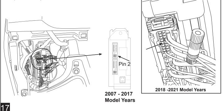
Locate 20 pin connector at bottom of panel on left. Connect blue Power Step wire to 18 gage blue wire *(Driver Front)* in pin 15 of connector shown. Plugs are located to the left of E Brake Pedal.
