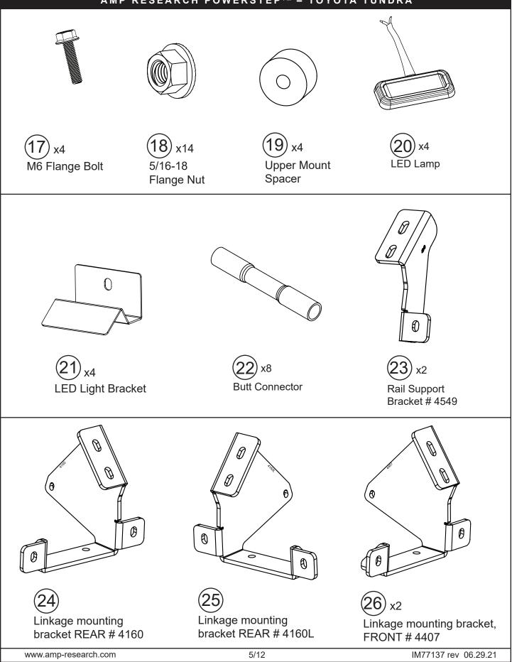
Install Front linkage mounting bracket (#26) (part# 4407 Front) using supplied Conical Washer bolts (#10). Use second set of mounting holes from front. Do not tighten to allow for adjustment. Take note of bracket orientation.
