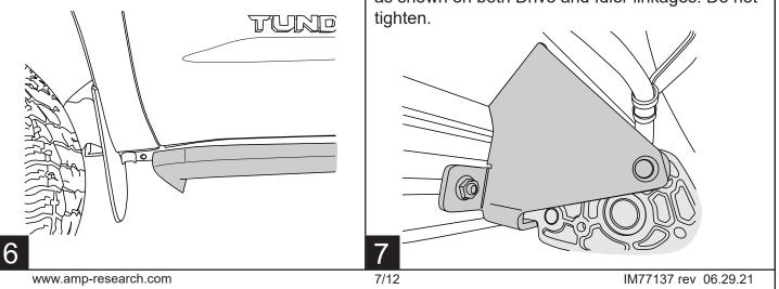
Slide mounting T-nut into position. Center Board in rail pocket. Tighten fasteners to 10ft-lb.
