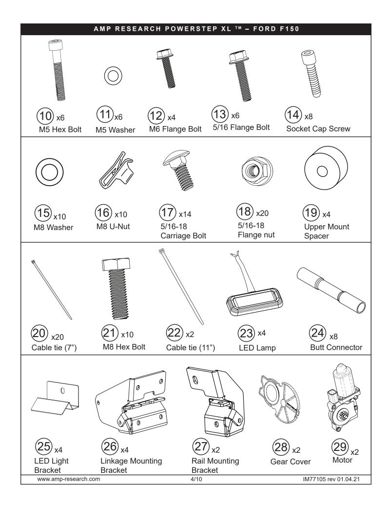
Insert 7 Carriage bolts (17) into slot on rail (4). Insert from either end of rail. Add 2 Light Brackets (25) on the 3rd and 5th bolt. Insert Flange nut (18) onto bracket tab to attach light brackets into position shown. Leave loose to allow for adjustment.
