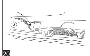
Pull wires from grommet and route back along factory wire harness to back door sill plate.
