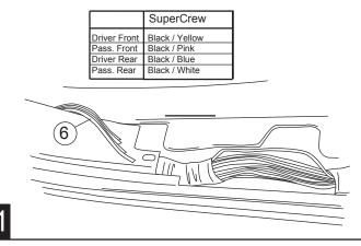
Using supplied Posi-Taps<sup>™</sup>, splice Power Step trigger wires into the corresponding door ajar wires. The SuperCrew (having 4 independent doors) is the only application that will use all four wires; tape off the two unused trigger wires on the SuperCab and Regular Cab.
