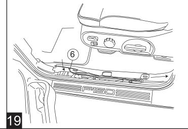
Locate the appropriate signal wires as noted below. Note: There may be up to five Black with Blue Stripe wires; use the one that looks unique (ie. different blue stripe... weight and shade).
