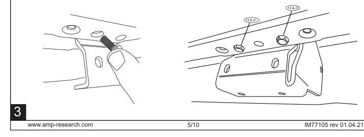
Using provided captive washer m8 bolts (8) install upper bracket hardware to brackets. Do not tighten.
