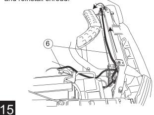
Puncture grommet and thread all four trigger wires up into the cabin of vehicle. The grommet is located on driver-side behind forward linkage assembly.
