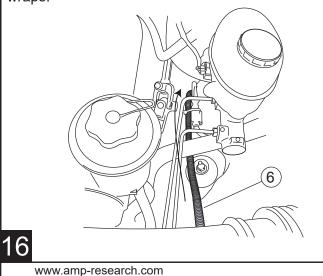
Mount controller with the two 11" tie wraps to factory conduit. Route wire harness under core support and down toward controller. Attach harness to controller (make sure connector locking tabs fully engage).
