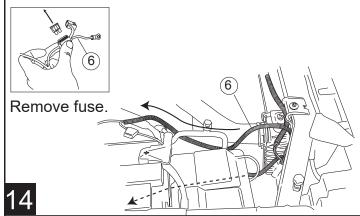
Route longer leg of harness down along driver-side wheel well and along frame of vehicle. Secure with tie wraps.
