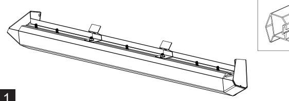
Locate mounting points. Frist middle and last set of holes on the inner sill. Install 5 U-nuts (16) in upper mount holes.
