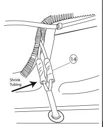
Close and wrap with conduit and electrical tape. Secure all loose wires with cable ties with lamp wires pulled upward to avoid any wire snagging.
