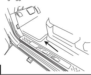
Remove grommet in floor panel above front linkage on driver side. Poke small hole into grommet and thread the two trigger wires through and up into the cabin of vehicle. Seal grommet with silicone sealer.
