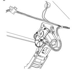
Remove driver side front kick panel and door sill plate. Roll back carpet to access hole for passing trigger wires into cab of vehicle.
