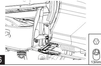
Center step pad on lower mount and scure using provided PT Screws. Tighten to 5ft-lbs using a T25 Torx bit. Verify Step pad alignment to body line of vehicle. Once step pad is in line to vehicle torque all bracket hardware to 16ft-lbs.
