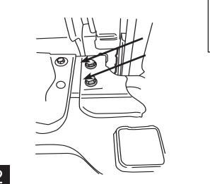
Install bracket to truck Torque nuts to 59 ft-lbs / 80Nm
