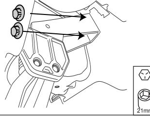
Insert threaded bracket into bumper and assemble bracket with supplied bolt. **Use** slotted end of bracket at bolt.
