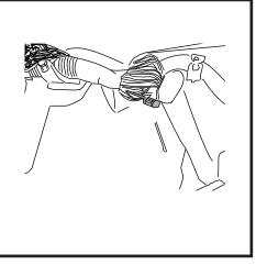
Measure from the front edge of door line on the pinch weld to the specified lengths below. Measure at 12" for the front LED Light and 60" for the rear LED Light.
