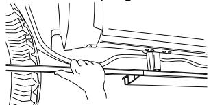
Once Trim Strip is installed verify that it is properly engaged along the Running Board.
