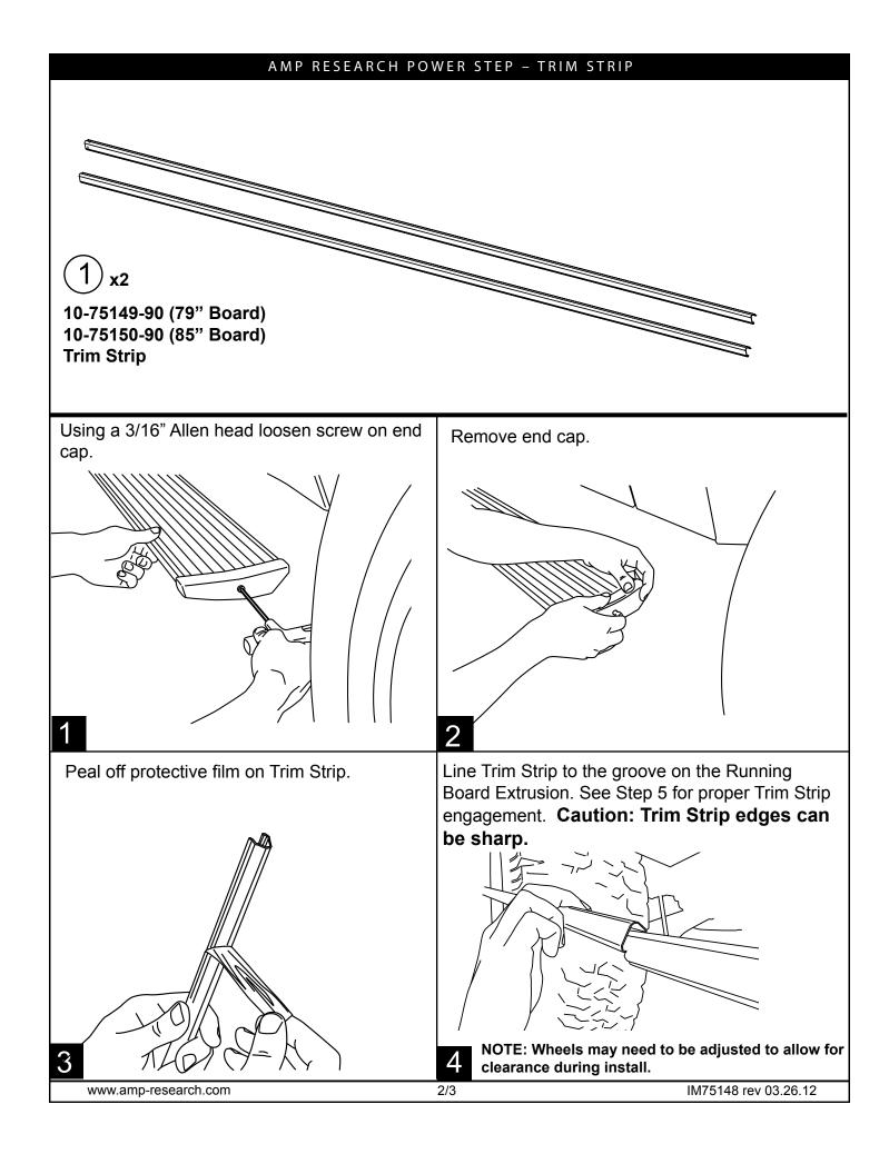
NOTE: Trim Strip should be lined up in both the upper and lower grooves.
