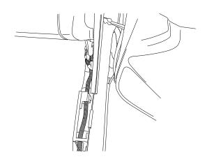
Install Single Diode harness as shown in step 21 on Pink/Black wire (12 volt negative with door open) and connect to Power Step Pink/Black trigger wire. Make sure to install the diode toward the front of the vehicle.
