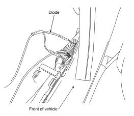
Connect wire harness to motor. Slide rubber grommet on Wire Harness into slot of Motor Cover. Slide Motor Cover over Motor. Insert plastic push pin rivets in mounting holes of motor cover
