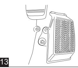
Pull up carpet and locate rubber grommet. Slice the grommet and pass trigger wires from under the vehicle and into the cab.
