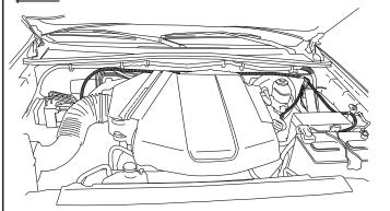
Note: Run loom with Green/Yellow and Pink/ 2 Black Trigger wires down drivers side of vehicle.
