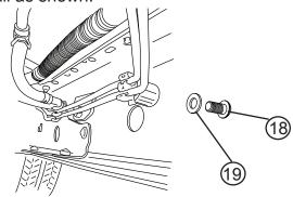
Replace all brake line fasteners.
