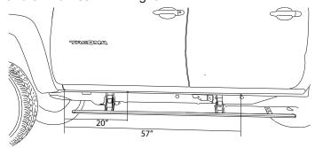
Drill a pilot hole followed by a 9/32" hole through the pinch weld at marked locations. Debur all holes.
