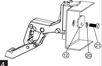
Through-bolt linkage to frame as shown in next step.
