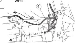
Route longer leg of harness across front and down under driver side. Secure harness with tie wraps and reinstall shroud.
