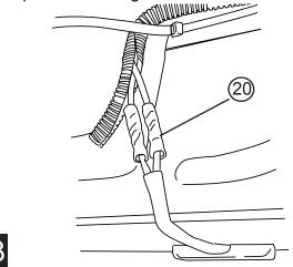
Close and wrap with conduit and electrical tape. Secure all loose wires with cable ties, with lamp wires pulled upward to avoid any wire snagging.
