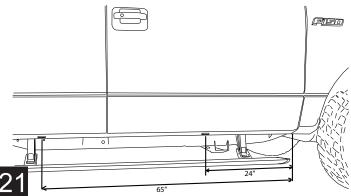
Affix lamps to rocker panel surface. Make sure the lamp is affixed to a clean, flat surface. There is a step down midway across the surface. Affix lamp just outside of step down.
