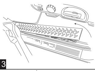
Pull wires from grommet and route back along factory wire harness to back door sill plate.
