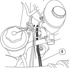
Puncture grommet and thread all four trigger wires up into the cabin of vehicle. The grommet is located on driver-side behind forward linkage assembly.
