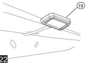
Using supplied butt connectors, connect the lamp wires. Red to Red, Black to Black. Once Crimped use heat gun to shrink tube.
