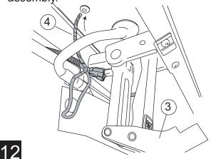
Remove drivers-door sill plate and pull back carpet to reveal trigger wires threaded though grommet.
