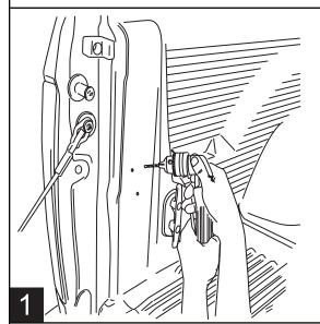
Using a power drill and 9/64" drill bit, drill through the existing dimple holes in sheet metal. If equipped with a bedliner, drill through bedliner.
