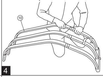
Adjust the width of the BEDXTENDER to fit the preinstalled mounting brackets. To keep tube overlap constant, adjust each tube so that the gap between the edge and the tape is the same.
