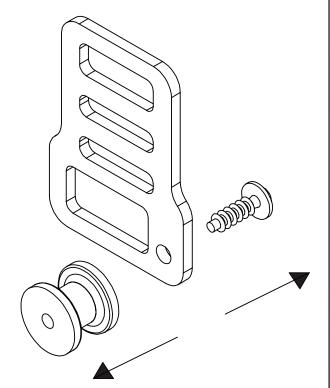
Install Strap Buckle Insert with the provided 10/32 x 7mm socket head cap screw with a 4mm hex key. Repeat for other strap.
