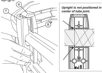
NOTE: The inside of the upright is stepped to fit correctly around the small and large diameter tubes.
