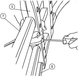
NOTE: Do not over tighten as this may strip out. Fastener will reach a noticable stopping point.
