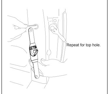
Once both hold down brackets are in place, pull on the mounting bracket assembly to position the hold down brackets. Make sure that the protrusions on the hold down bracket engage themselves with the edge of the hole
