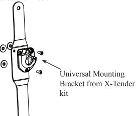
Pass button head bolt through internal tooth washer, mounting bracket and hold down bracket and engage with nut.
