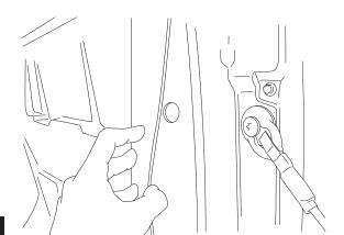
Mark hole position on bedliner for both top and bottom holes and center punch to make a drill guide.
