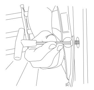
Repeat for lower hole. Torque to 5 ft.lbs. Repeat steps 1-8 for vehicles without bedliner and steps 9-14 for vehicles with bedliner on other side.
