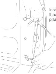
Insert hold down bracket through lower hole of the bed pillar.
