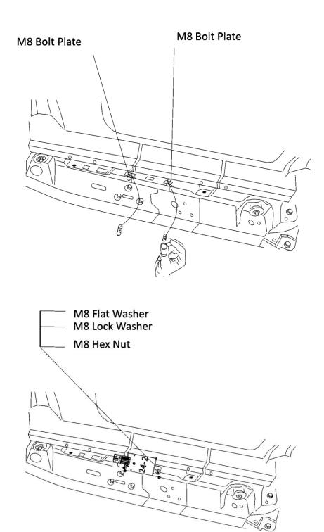
**Step 8**: Locate the paired square holes in the center of the body and insert the M8 bolt plates inside.
