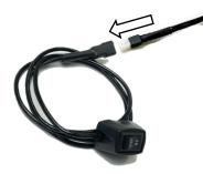
**Step 23:** Locate the black wires for the disable switch and feed them to your desired mount location. Prepare the surface by cleaning with a 50/50 mix of isopropyl alcohol and water or equivalent. Once the surface is dry, peel the backing from the double-sided tape and stick the disable switch on the lower dash panel. Plug the disable switch connector into the black wire harness and tuck the extra wire behind the lower dash panel.
