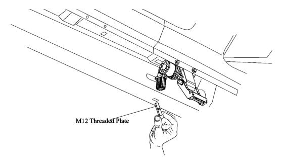
**Step 6**: Locate elongated hole opening on the front of the frame (before the body mount) and insert the M12 threaded plate and align thread with hole on the bottom side of the frame.
