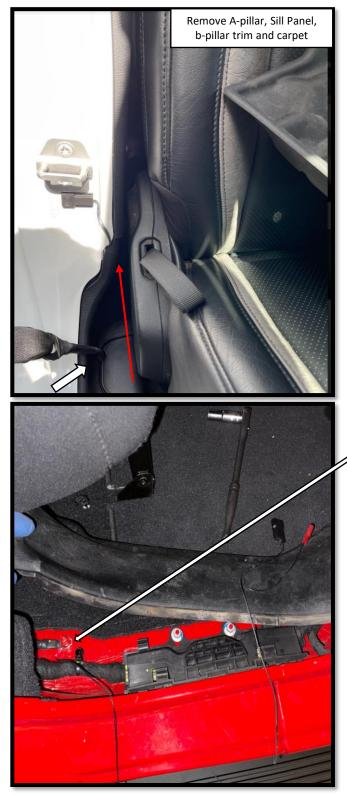
**Step 19:** Route the passenger side door trigger wire (brown) towards the passenger side b-pillar. Route the driver side door trigger wire (white) and the black disable switch wires under the center console to the left side of the vehicle. The white wire needs to go to the driver side b-pillar, the black wires will go to the center console.
