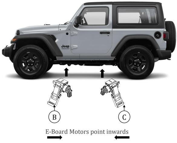
**Step 12**: Repeat Steps 1-11 to install the motor linkage assemblies and running board on the driver side.
