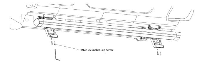
**Step 10**: Install the Passenger side running board. With assistance, begin by positioning the board on the front and rear motor assembly bases. Align the sliding T-Nut on the running board with the slots on the front and rear motor base. Once the T-Nuts are aligned, rotate the running board so that the T-Nuts set in the slots on the base of the arms. Repeat 1-14 to install the motor linkage assemblies and running board on the driver side side.
