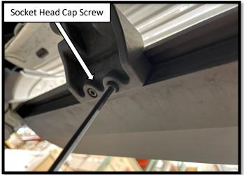
**Step 11**: Determine where you want to position the board and secure the running board to the arms using the (2 per bracket) M6x25 socket head cap screws. Using a torque wrench, tighten to 9 ft-lbs. Step # With the running board is installed, fasten the hardware on the Passenger side front and rear motor assemblies. Using a torque wrench, tighten the mounting hardware to 18 ft-lbs.
