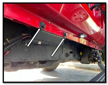
**Step 9**: Using the middle two holes on the pinch seam below the passenger side front door. Using two M8 hex head bolts, M8 flat washers and M8 lock washers, install the controller mounting bracket. Using a torque wrench, tighten to 18 ft-lb.
