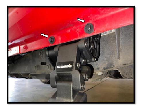
Step 5: Install the front passenger side motor using (2) M8X35mm Hex Bolts, (2) M8 lock washer, (2) M8 flat washer to fasten the motor to the vehicle. The hardware should be hand tightened only until snug. This will allow the motor assembly to move and align easier when installing the running board.
