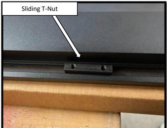
**Step 10**: Install the Passenger side running board. With assistance, begin by positioning the board on the front and rear motor assembly bases. Align the sliding T-Nut on the running board with the slots on the front and rear motor base. Once the T-Nuts are aligned, rotate the running board so that the T-Nuts set in the slots on the base of the arms. Repeat 1-14 to install the motor linkage assemblies and running board on the driver side side.
