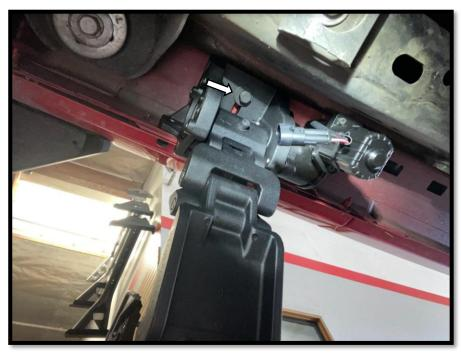
Step 6: Underneath the front passenger side motor install (1) M8X35mm Hex Bolts, (1) M8 lock washer, (1) M8 flat washer. The hardware should be hand tightened only until snug. This will allow the motor assembly to move and align easier when installing the running board.
