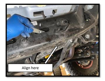
**Step 7**: Locate elongated hole opening on the front of the frame (before the body mount) and insert the M12 threaded plate and align thread with hole on the bottom side of the frame.
