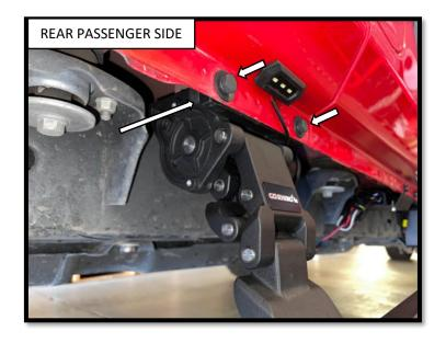
**Step 3**: Install the rear PASSENGER side motor using (2) M8X35mm Hex Bolts, (2) M8 lock washer, (2) M8 flat washer and (1) REAR MOUNTING BASE PLATE SPACER to fasten the motor to the vehicle. The hardware should be hand tightened only until snug. This will allow the motor assembly to move and align easier when installing the running board.
