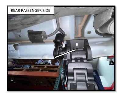
**Step 4**: Underneath the rear passenger side motor install (1) M8X35mm Hex Bolts, (1) M8 lock washer, (1) M8 flat washer. The hardware should be hand tightened only until snug. This will allow the motor assembly to move and align easier when installing the running board.
