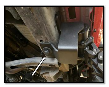
**Step 8**: Install the passenger side front motor protective bracket. Secure the protective bracket using an M12 hex bolt, flat washer, and lock washer. Torque to 25 ft-lbs.
