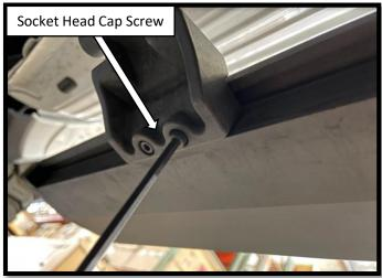
**Step 8**: Determine where you want to position the board and secure the running board to the arms using the (2 per bracket) M6x25 socket head cap screws. Using a torque wrench, tighten to 9 ftlbs. Step # With the running board is installed, fasten the hardware on the Passenger side front and rear motor assemblies. Using a torque wrench, tighten the mounting hardware to 18 ftlbs.
