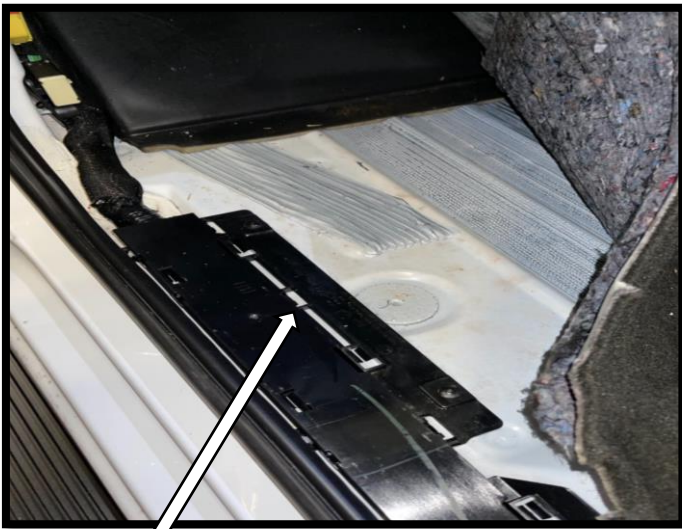
Driver Side carpet, pull back to expose grommet opening
