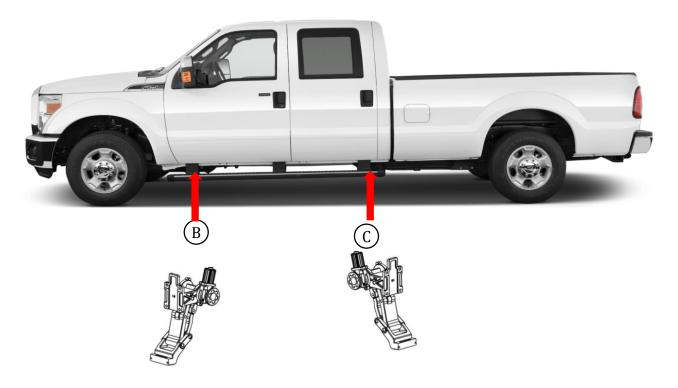
**Step 10**: Repeat Steps 2-7 to install the motor linkage assemblies. Repeat steps 8-9 to install running board on the Driver side.
