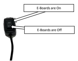
**Step 24:** Open the Driver side door and keep the door open. Flip the disable switch to the Off position. This will signal the running boards to retract to the stowed position and it will disable any further operation until the switch is flipped to the On position.
