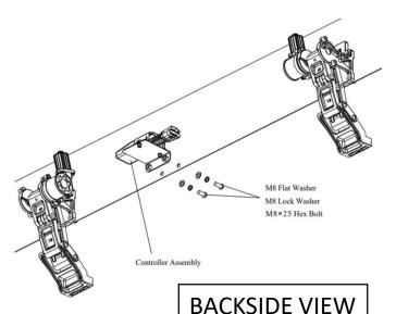
**Step 7**: Install the Controller Assembly on the passenger side center mounting location using (2) Mhex bolts, (2) M8 Flat Washers, (2) M8 Lock Washers into the front mounting holes of the pinch weld to fasten the motor to the truck. The hardware should be hand tightened only until snug. This will allow the motor assembly to move and align easier when installing the running board.
