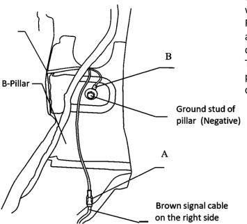
**Step 15:** Route the passenger side door trigger wire (brown) towards the driver side b-pillar. Route the driver side door trigger wire (white) and the black disable switch wires under the center console to the left side of the vehicle. The white wire needs to go to the driver side b-pillar, the black wires will go to the center console.
