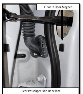
Step 19: REAR DOOR Apply a vertically oriented strip of masking tape on the front driver side door using the deepest part of the latch as a reference point. Make a mark 2-3" below the center line of the latch. Prepare the surface by cleaning with a 50/50 mix of isopropyl alcohol and water or equivalent. Once the surface is completely dry, peel the backing from the double-sided tape and stick the magnet to the door. Align the top of the magnet with the 5" mark as shown.
