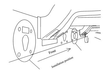
**Step 3**: Install the front Passenger side motor using (2) hex bolts, (2) M8 Flat Washers, (2) M8 Lock Washers and (2) M8 Spring into the upper mounting holes of the rocker panel to fasten the motor to the truck. The hardware should be hand tightened only until snug. This will allow the motor assembly to move and align easier when installing the running board.
