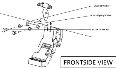
**Step 6**: Install the Rear Passenger side motor using (2)M10 hex bolts, (2) M10 Flat Washers, (2) M10 Lock Washers into the front mounting holes of the pinch weld to fasten the motor to the truck. The hardware should be hand tightened only until snug. This will allow the motor assembly to move and align easier when installing the running board.
