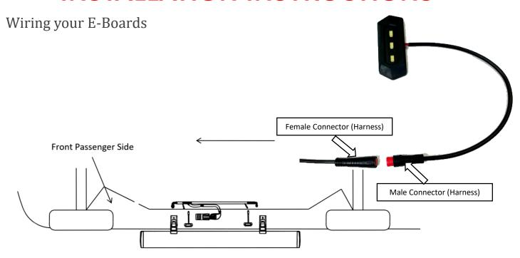
**Step 12**: Align the arrows on the small round connectors and plug the PASSENGER side front and PASSENGER side rear LED lights. Prepare the surface by cleaning with a 50/50 mix of isopropyl alcohol and water or equivalent. Once the surface is completely dry, peel the backing from the double-sided tape and stick the LEDs to the bottom side of the rocker panel. Position the LED lights at the center of the front and rear passenger side doors
