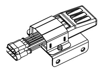
**Notice:** As shown in the picture, there is a four conductor plug, a six-conductor plug, a black two conductor plug, and a red two-conductor plug.
