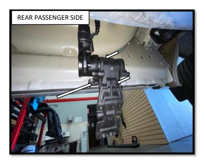
**Step 3**: Install the rear PASSENGER side motor on the 3 threaded studs located on the inside rocker panel towards the rear of cab using (3) M8 Hex Nuts, (3) M8 Flat Washers and (3) M8 Lock Washers. The hardware should be hand tightened only until snug. This will allow the motor assembly to move and align easier when installing the running board.
