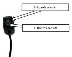
**Step 23:** Open the Driver side door and keep the door open. Flip the disable switch to the Off position. This will signal the running boards to retract to the stowed position and it will disable any further operation until the switch is flipped to the On position.
