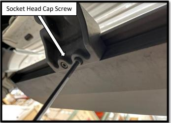
**Step 6**: Determine where you want to position the board and secure the running board to the arms using the (2 per bracket) M6x25 socket head cap screws. Using a torque wrench, tighten to 9 ft-lbs. With the running board installed, fasten the hardware on the Passenger side front and rear motor assemblies. Using a torque wrench, tighten the mounting hardware to 18 ft-lbs.
