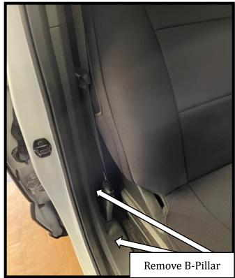
**Step 14:** Route the passenger side door trigger wire (brown) towards the passenger side bpillar. Route the driver side door trigger wire (white) and the black disable switch wires under the center console to the left side of the vehicle. The white wire needs to go to the driver side b-pillar, the black wires will go to the center console.
