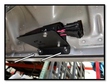
**Step 4**: Install the controller module on the two threaded studs located near the center of cab on the passenger side rocker panel using (2) M8 Hex Nuts, (2) M8 Flat Washers and (2) M8 Lock Washers. Using a torque wrench, tighten to 18 ft-lb
