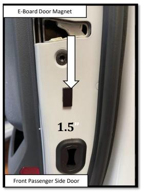
Step 16: FRONT DOOR Apply a vertically oriented strip of masking tape on the front Passenger side door using the deepest part of the latch as a reference point. Make a mark 1.5" below the center line of the latch. Prepare the surface by cleaning with a 50/50 mix of isopropyl alcohol and water or equivalent. Once the surface is completely dry, peel the backing from the double-sided tape and stick the magnet to the door. Align the top of the magnet with the 1.5" mark as shown.
