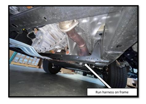
**Step 11**: Route the motor and LED wire harness from the controller to the DRIVER side frame rail of the vehicle. When routing the harness keep clear from any moving parts and avoid direct contact with the exhaust system.
