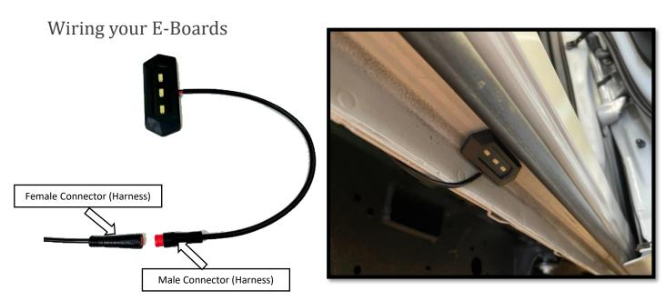
**Step 10**: Align the arrows on the small round connectors and plug the Passenger side front and Passenger side rear LED lights. Prepare the surface by cleaning with a 50/50 mix of isopropyl alcohol and water or equivalent. Once the surface is completely dry, peel the backing from the double-sided tape and stick the LEDs to the bottom side of the rocker panel. Position the LED lights at the center of the front and rear passenger side doors
