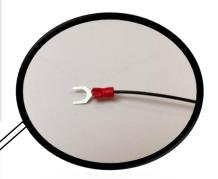
**Step 15:** The door trigger sensor harness will need a ground connection to the vehicle. Locate the seat belt assembly at the passenger side b-pillar and install the ground wire under the top bolt of the seat belt assembly.
