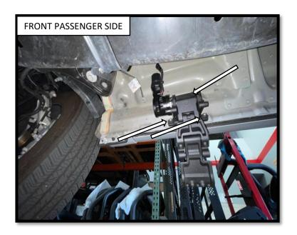
**Step 4**: Install the front PASSENGER side motor on the 3 threaded studs located on the inside rocker panel towards the rear of cab. using (3) M8 Hex Nuts, (3) M8 Flat Washers and (3) M8 Lock Washers. The hardware should be hand tightened only until snug. This will allow the motor assembly to move and align easier when installing the running board.
