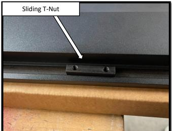
**Step 5**: Install the Passenger side running board. With assistance, begin by positioning the board on the front and rear motor assembly bases. Align the sliding T-Nut on the running board with the slots on the front and rear motor brackets. Once the T-Nuts are aligned, rotate the running board so that the T-Nuts set in the slots on the base of the arms.
