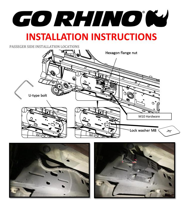
**Step 5**: Locate the hole near the center of the cab on the Passenger side frame of the vehicle. Insert the bolt plate into the elongated hole and secure it using the M8 plastic washer. Position the control module against the bolt plate and secure using (2) M8 nuts, flat washer and lock washer.
