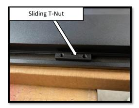
**Step 6**: Install the passenger side running board. With assistance, begin by positioning the board on the front and rear motor assembly bases. Align the sliding T-Nut on the running board with the slots on the front and rear motor base. Once the T-Nuts are aligned, rotate the running board so that the T-Nuts set in the slots on the base of the arms. Repeat Steps 3-6 to install the motor linkage assemblies and running board on the Driver side.
