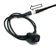
**Step 21:** Locate the black wires for the disable switch and feed them to your desired mount location. Prepare the surface by cleaning with a 50/50 mix of isopropyl alcohol and water or equivalent. Once the surface is dry, peel the backing from the double-sided tape and stick the disable switch on the lower dash panel. Plug the disable switch connector into the black wire harness and tuck the extra wire behind the lower dash panel.
