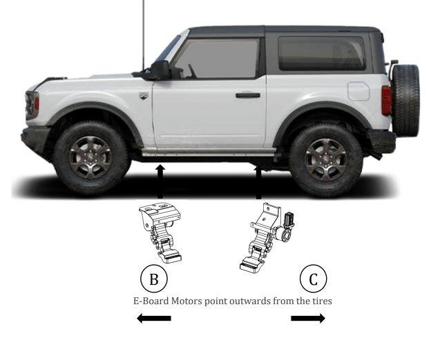
**Step 8**: Repeat Steps 1-4 to install the motor linkage assemblies on the passenger side. Repeat steps 6-7 to install running board on the driver side.
