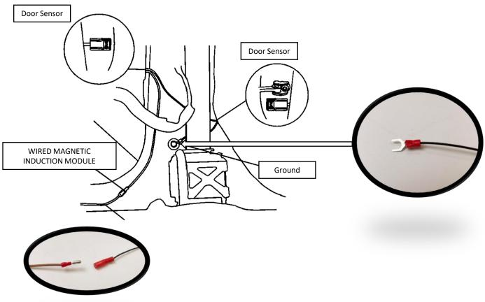
**Step 14:** The door trigger sensor harness will need a ground connection to the vehicle. Locate the seat belt assembly at the driver side b-pillar and install the ground wire under the top bolt of the seat belt assembly. Connect the snap-in bullet connector to the brown wire on the Passenger side b-pillar.
