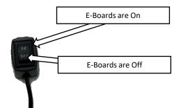
**Step 23:** Open the PASSENGER side door and keep the door open. Flip the disable switch to the Off position. This will signal the running boards to retract to the stowed position and it will disable any further operation until the switch is flipped to the On position.
