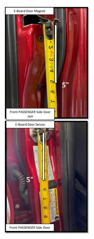
**Step 16: FRONT DOOR** Apply a vertically oriented strip of masking tape on the front PASSENGER side door using the deepest part of the latch as a reference point. Make a mark 5" below the center line of the latch. Prepare the surface by cleaning with a 50/50 mix of isopropyl alcohol and water or equivalent. Once the surface is completely dry, peel the backing from the double-sided tape and stick the magnet to the door. Align the top of the magnet with the 5" mark as shown.
