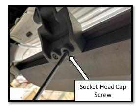
**Step 7**: Determine where you want to position the board and secure the running board to the arms using the (2 per bracket) M6x25 socket head cap screws. Using a torque wrench, tighten to 9 ft-lbs. Step # With the running board is installed, fasten the hardware on the Driver side front and rear motor assemblies. Using a torque wrench, tighten the mounting hardware to 18 ft-lbs.
