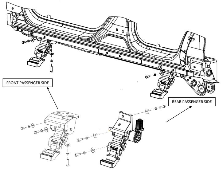
**Step 3**: Install the front passenger side motor using (2) M8x25MM hex bolts , (2) M8 Lock Washer, (2) M8 Flat Washer on the pinch weld and (1) M10x35MM hex bolts , (1) M10 Lock Washer, (1) M10 Flat Washer on the rocker panel, to fasten the motor to the vehicle. The hardware should be hand tightened only until snug. This will allow the motor assembly to move and align easier when installing the running board.
