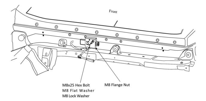
**Step 3**: Install CONTROL MODULE(1) hex bolts, (1) M8 Flat Washers, (1) M8 Lock Washers and (1) M8 Spring into the bottom mounting holes of the rocker panel to fasten the motor to the truck. Install (1) M8 Flange nut on the upper mounting hole of the rocker panel. The mounting location is on the center of the rocker panel.
