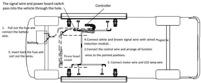
**Step 13**: Route the motor and LED wire harness from the controller to the Driver side frame rail of the vehicle. When routing the harness keep clear from any moving parts and avoid direct contact with the exhaust system.
