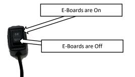
**Step 24:** Open the Driver side door and keep the door open. Flip the disable switch to the Off position. This will signal the running boards to retract to the stowed position and it will disable any further operation until the switch is flipped to the On position.
