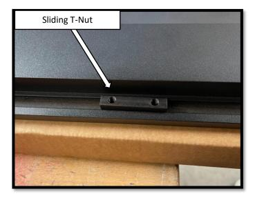
**Step 8**: Install the driver side running board. With assistance, begin by positioning the board on the front and rear motor assembly bases. Align the sliding T-Nut on the running board with the slots on the front and rear motor base. Once the T-Nuts are aligned, rotate the running board so that the T-Nuts set in the slots on the base of the arms.
