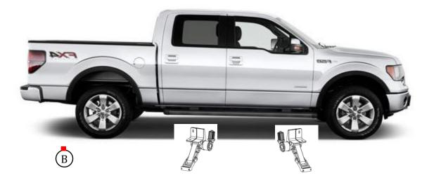
**Step 10**: Repeat Steps 2-7 to install the motor linkage assemblies. Repeat steps 8-9 to install running board on the Driver side.
