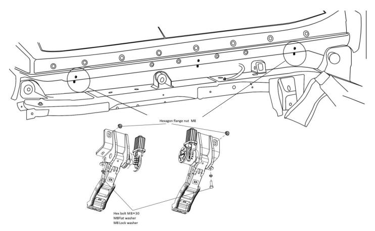
**Step 3**: Install BOTH Driver side motors using (1) hex bolts, (1) M8 Flat Washers, (1) M8 Lock Washers and (2) M8 Spring into the bottom mounting holes of the rocker panel to fasten the motor to the truck. Install M8 Flange nut on the upper mounting hole of the rocker panel. The hardware should be hand tightened only until snug. This will allow the motor assembly to move and align easier when installing the running board.
