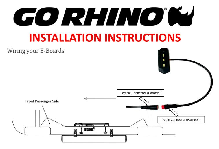
**Step 12**: Align the arrows on the small round connectors and plug the PASSENGER side front and PASSENGER side rear LED lights. Prepare the surface by cleaning with a 50/50 mix of isopropyl alcohol and water or equivalent. Once the surface is completely dry, peel the backing from the double-sided tape and stick the LEDs to the bottom side of the rocker panel. Position the LED lights at the center of the front and rear passenger side doors
