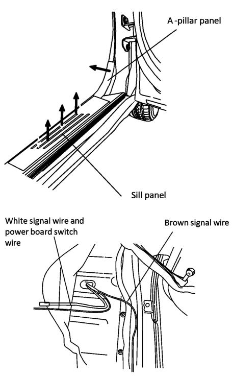
**Step 14:** On the Passenger side, remove the front kick panel, front door sill trim panel, and b-pillar trim panel. Pull the front passenger carpet back and cut a 7/16" hole on the rubber gromet as shown. Feed the door trigger signal wires (white and brown) and the disable switch wires (two black wires) into the cab. Seal around the wires using RTV silicone adhesive to prevent water intrusion.
