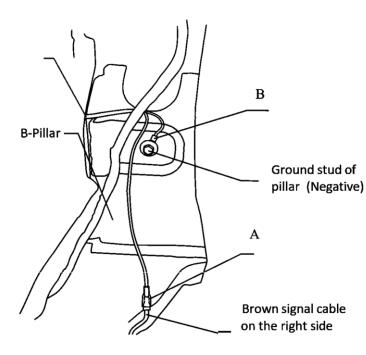
**Step 15:** Route the passenger side door trigger wire (brown) towards the driver side b-pillar. Route the driver side door trigger wire (white) and the black disable switch wires under the center console to the left side of the vehicle. The white wire needs to go to the driver side b-pillar, the black wires will go to the center console.
