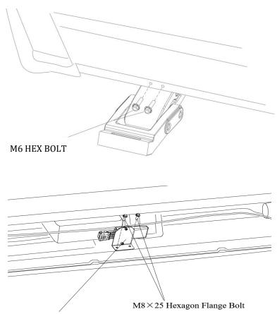
**Step 5**: Install the rear and front Driverside motor using two M6 flange bolts to fasten the motor to the pinchseam. The hardware should be hand tightened only until snug. This will allow the motor assembly to move and align easier when installing the running board.
