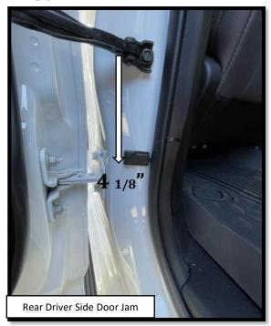
**Step 19:** REAR DOOR: With the weatherstrip peeled back, route the sensor wire underneath it. Clean the surface by cleaning with a 50/50 mix of isopropyl alcohol and water or equivalent. Once the surface is completely dry, peel the backing from the double-sided tape and stick the sensor on the door jamb. Align the top of the sensor with the 4 1/8"
