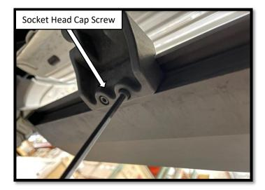
**Step 8**: Determine where you want to position the board and secure the running board to the arms using the (2 per bracket) M6x25 socket head cap screws. Using a torque wrench, tighten to 9 ft-lbs. Step # With the running board is installed, fasten the hardware on the Driver side front and rear motor assemblies. Using a torque wrench, tighten the mounting hardware to 18 ft-lbs.
