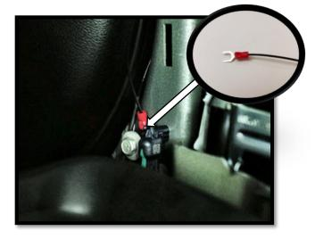
**Step 16:** The door trigger sensor harness will need a ground connection to the vehicle. Locate the hex head screw near the seatbelt assembly and install the ground under the plastic housing as shown.
