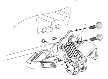
**Step 4**: Install the rear Driver side motor using (1) Nut Plate , (2) M8 Hex Bolts. Holes that donothave factory threaded inserts will require the threaded nut bracket that is included in this kit. The hardware should be hand tightened only until snug. This will allow the motor assembly to move and align easier when installing the running board.
