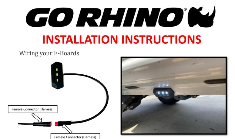
**Step 12**: Align the arrows on the small round connectors and plug the Driver side front and Driver side rear LED lights. Prepare the surface by cleaning with a 50/50 mix of isopropyl alcohol and water or equivalent. Once the surface is completely dry, peel the backing from the double-sided tape and stick the LEDs to the bottom side of the rocker panel. Stick the LED lights at the center of the front and rear Driver side doors
