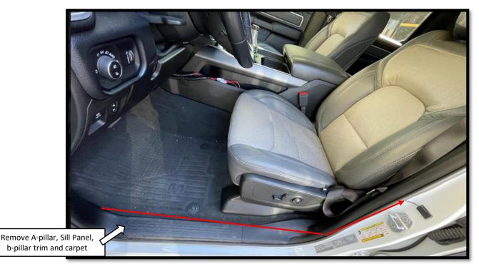
**Step 15:** Route the Driver side door trigger wire (brown) towards the Driver side b-pillar. Route the Passenger side door trigger wire (white) under the center console and over to the Passenger side b-pillar. Route the black disable switch wires to the center console.
