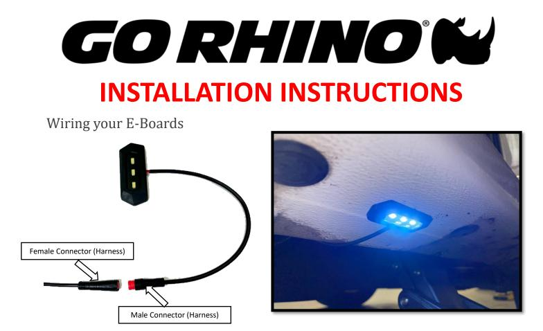
**Step 10**: Align the arrows on the small round connectors and plug the Passenger side front and Passenger side rear LED lights. Prepare the surface by cleaning with a 50/50 mix of isopropyl alcohol and water or equivalent. Once the surface is completely dry, peel the backing from the double-sided tape and stick the LEDs to the bottom side of the rocker panel. Position the LED lights at the center of the front and rear passenger side doors
