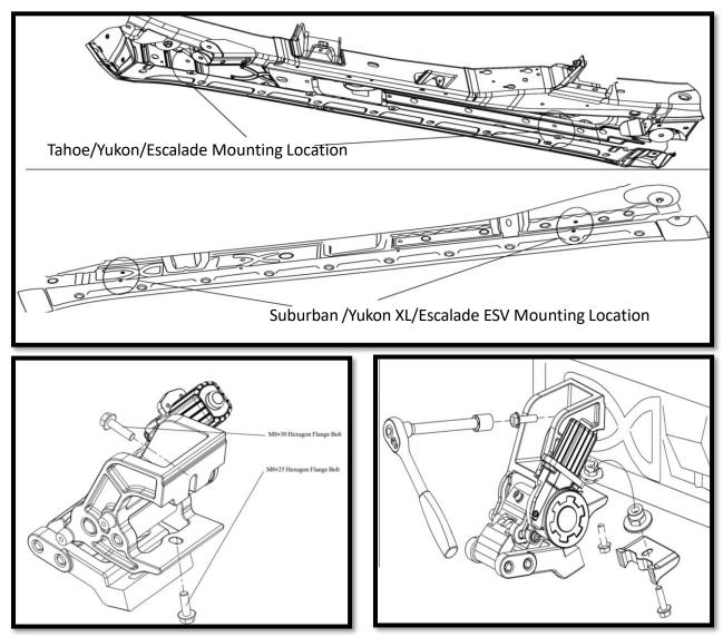
**Step 3:** Install front Passenger and rear Passenger side motor using M8x30 Hex Flange Bolt on the top mounting hole and M8x25 on the bottom mounting hole. Use M8 Flat washer and M8 Hex nut on the bottom mounting hole.
