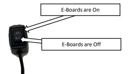
**Step 21:** Open the Driver side door and keep the door open. Flip the disable switch to the Off position. This will signal the running boards to retract to the stowed position and it will disable any further operation until the switch is flipped to the On position.
