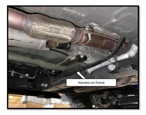
**Step 11**: Route the motor and LED wire harness from the controller to the Driver side frame rail of the vehicle. When routing the harness keep clear from any moving parts and avoid direct contact with the exhaust system.
