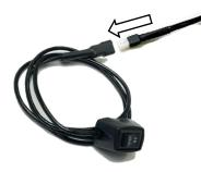
**Step 19:** Locate the black wires for the disable switch and feed them to your desired mount location. Prepare the surface by cleaning with a 50/50 mix of isopropyl alcohol and water or equivalent. Once the surface is dry, peel the backing from the double-sided tape and stick the disable switch on the lower dash panel. Plug the disable switch connector into the black wire harness and tuck the extra wire behind the lower dash panel.
