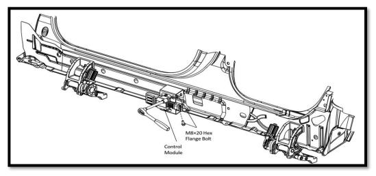
**Step 4:** Install the control module on the center passenger side mounting provision using M8x20 Hex Flange Bolt on the top mounting holes (2)
