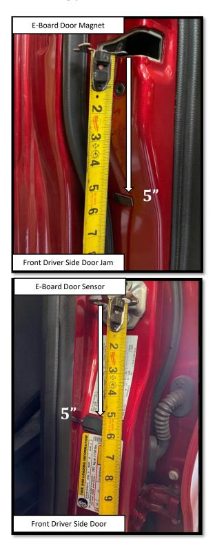
**Step 17: FRONT DOOR** Apply a vertically oriented strip of masking tape on the front driver side door using the deepest part of the latch as a reference point. Make a mark 5" below the center line of the latch. Prepare the surface by cleaning with a 50/50 mix of isopropyl alcohol and water or equivalent. Once the surface is completely dry, peel the backing from the double-sided tape and stick the magnet to the door. Align the top of the magnet with the 5" mark as shown.
