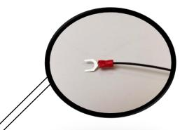
**Step 16:** The door trigger sensor harness will need a ground connection to the vehicle. Locate the seat belt assembly at the driver side b-pillar and install the ground wire under the top bolt of the seat belt assembly.
