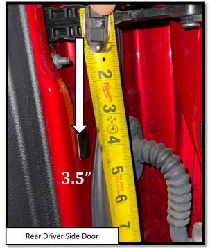
**Step 20:** With the rear driver side sensor attached, you can determine the correct position for the door magnet. peel the backing from the double-sided tape and stick the magnet on the door. Align the bottom of the magnet with the 3.5"
