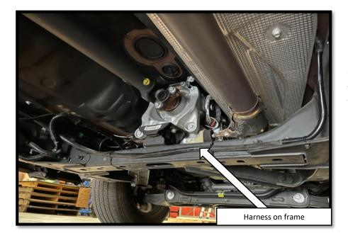
**Step 13**: Route the motor and LED wire harness from the controller to the Passenger side frame rail of the vehicle. When routing the harness keep clear from any moving parts and avoid direct contact with the exhaust system.
