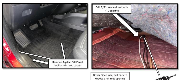
Driver Side Liner, pull back to expose grommet opening
