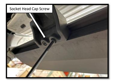
**Step 9**: Determine where you want to position the board and secure the running board to the arms using the (2 per bracket) M6x25 socket head cap screws. Using a torque wrench, tighten to 9 ft-lbs. Step # With the running board is installed, fasten the hardware on the Driver side front and rear motor assemblies. Using a torque wrench, tighten the mounting hardware to 18 ft-lbs.
