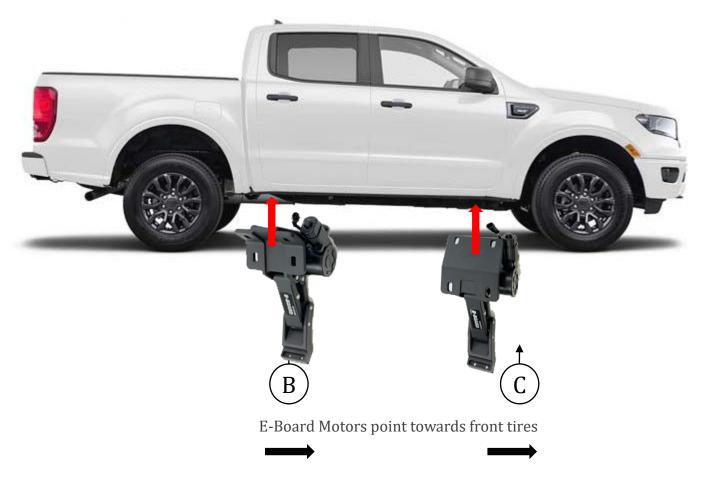
**Step 10**: Repeat Steps 2-6 to install the motor linkage assemblies. Repeat steps 8-9 to install running board on the Passenger side.
