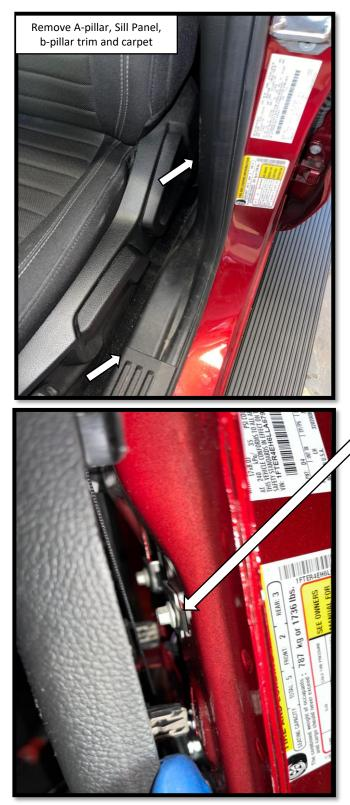
**Step 15:** Route the driver side door trigger wire (brown) towards the driver side b-pillar. Route the passenger side door trigger wire (white) and the black disable switch wires under the center console to the left side of the vehicle. The white wire needs to go to the passenger side b-pillar, the black wires will go to the center console.
