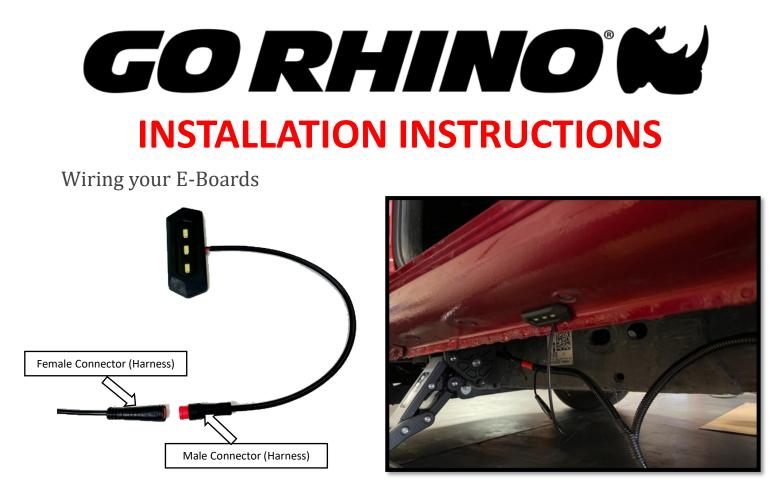
**Step 12**: Align the arrows on the small round connectors and plug the Driver side front and Driver side rear LED lights. Prepare the surface by cleaning with a 50/50 mix of isopropyl alcohol and water or equivalent. Once the surface is completely dry, peel the backing from the double-sided tape and stick the LEDs to the bottom side of the rocker panel. Position the LED lights at the center of the front and rear passenger side doors
