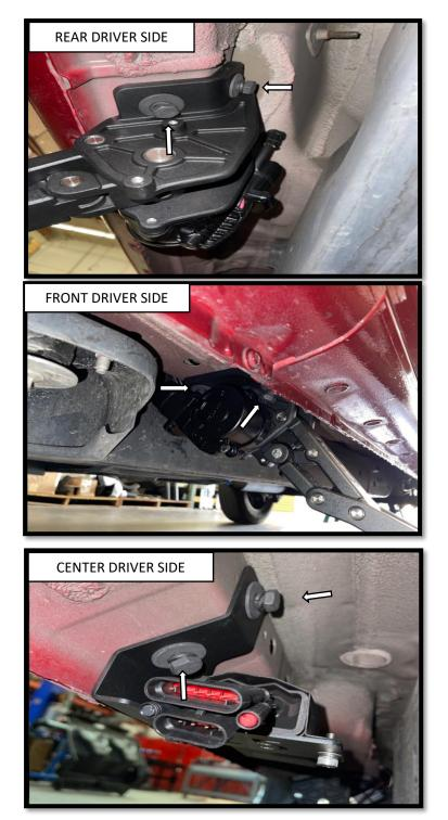
**Step 5**: Install the rear driver side motor using (2) M10x30MM hex bolts M10 Lock Washer, M10 Flat Washer, to fasten the motor to the truck. The hardware should be hand tightened only until snug. This will allow the motor assembly to move and align easier when installing the running board.
