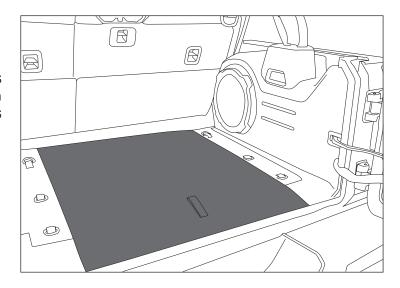
2. Remove passenger side tie downs using T40 Torx drive and remove carpeted panel.
