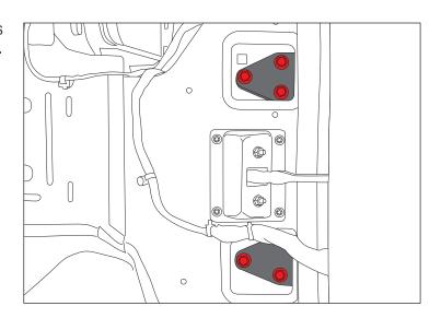
12. Insert Spartacus Hinge Casting in body openings and loosely install using six factory bolts removed in step 11.
