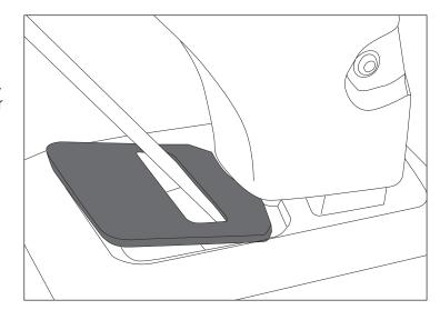
5. Remove screw by passenger side rear door using T25 Torx drive.
