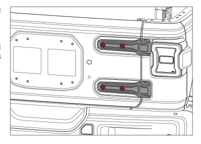
11. Without opening tailgate, remove six bolts securing factory hinges to body and remove hinges.
