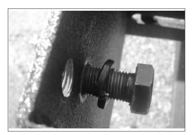
12. Slide the tire mounting hub over the adjustment hub as shown below. Using a supplied M12 x 30 bolt and washer, slide the bolt assembly through both the adjustment and tire mounting hubs. Place another washer over the bolt and thread on an M12 Nyloc nut. Repeat the above steps in the other 3 slots. Do not tighten the nuts
