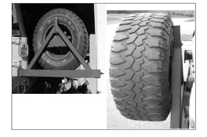
17. Close and latch the tire carrier. Insert and close lock pin.
