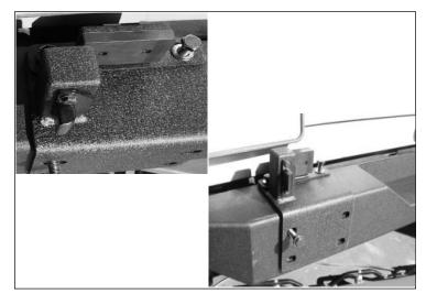
2. Attach catch post bracket to the bumper using a D-Ring. Place a D-Ring; the wider set of holes is the top of the D-Ring as shown below, against the catch post bracket, and insert an M12 x 60 bolt and washer through the top right corner of the D-Ring and loosely thread through. Remove the bolt installed in the top left corner and rotate the D-Ring into position and thread the remaining 3 bolts and washers into the D-Ring and sub-frames. Do
