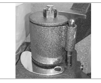
8. Place the 3rd brake light post over the opening in the top of the tire carrier and slide it in. With an M12 x 30 bolt and washer in hand, slide the brake post down, and insert the bolt and washer through one of the adjustment holes according to desired height. Tighten bolt.
