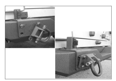
3. Place the tire carrier and spindle bracket on top of the bumper visually lining up the spindle bracket and bumper mounting holes. Thread 2 of the supplied M12 x 60 bolts and washers through the spindle bracket and bumper into the subframe. Do not tighten the bolts at this time.
