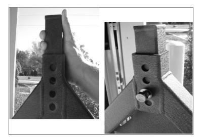
9. Open the tire carrier and place the adjustment hub up to tire carrier A-frame and align the 3 holes. Using 3 of the supplied M12 x 30 bolts and washers, insert through the tire carrier and the adjustment hub. Using 3 more washers and 3 Nyloc nuts, place the washers over the bolt and thread the Nyloc nuts onto the bolts. Tighten using a 3/4" wrench and 18mm socket and ratchet.
