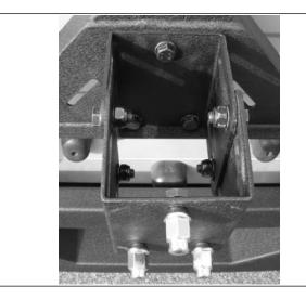
14. The tire carrier spindle assembly does come lightly lubricated from the factory;however, we recommend you lubricate the bearings of the spindle assembly with all purpose grease. Please refer to the model and pictures below for instruction on greasing the bearings of the tire carrier.
