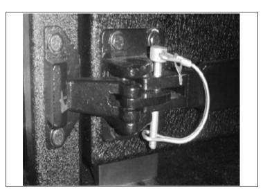
18. This completes the installation of the 1976-2006 XHD Tire Carrier. This product is designed to be maintenance free; however, due to the nature of the product, you should periodically check the condition of the tire carrier looking for abnormal wear or damage. Discontinue use if damage has occurred, or until proper repairs are made.
