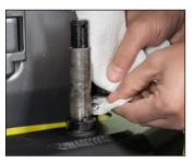
the housing (B). Install rubber seal to the bottom of housing (C), secure seal, may need to lightly tap with hammer. Install tire carrier over spindle. Install bearing (D). Next tighten castle nut (E). Tighten nut snug, back off a quarter turn. Swing tire carrier and assure it's secure. Tighten or loosen castle nut to desired feel. Insert cotter pin to secure castle nut. Install bearing cap (F).
