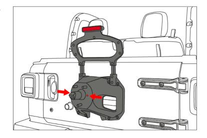
3. Using 13mm socket, remove eight factory bolts securing the spare tire mount. Remove wires for the third brake light and backup camera.
