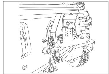
21. Reinstall the passenger side taillight. Requires the same procedure as step 10 in reverse. DO NOT overtighten plastic hardware, avoid damage to these plastic components.
