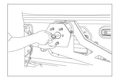
17. Slide the mount to the desired position according to the spare backspacing. This requires measuring the spare to determine the best position. Once in a position is determined, fully tighten all three bolts.
