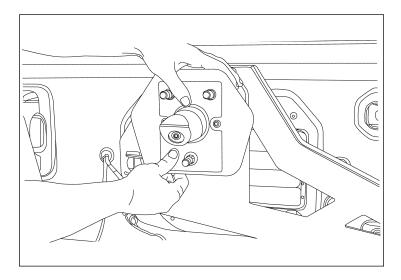
23. Install the spare tire to the carrier. With assistance, lift spare tire into position. Use the OE lug nuts to secure. Torque to 60 ft/lbs. We also suggest using a locking lug nut to assist against theft.
