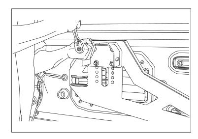
15. Place wheel stud bracket over the tire mount base. Use the three M12 X 35 bolts to attach with flat washers and Nylock nuts. The bolts install one at the top and two at the sides. **DO NOT fully tighten.**
