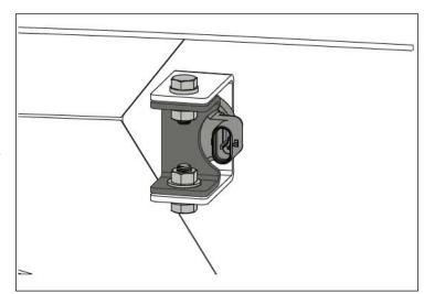
5. Install the passenger side nut plate into the passenger side frame rail. (Clean any dirt and debris) Make sure the nut plate sits flat and threaded nuts are accessible through the holes underneath the frame.
