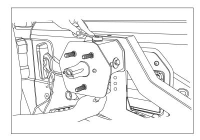
18. Route the backup camera wire through the tire carrier and wheel stud assembly. Plug-in camera, then attach using the three OE screws removed earlier.
