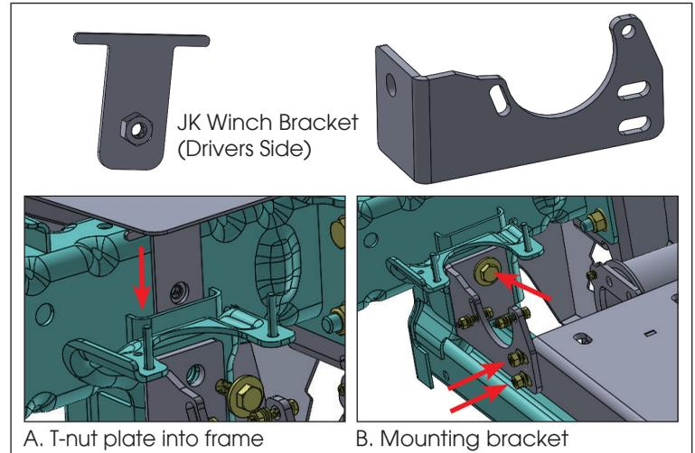
11. Now install passenger side JK winch bracket. Slide T-nut plate into the frame slot (see image A). The bracket mounts to the winch tray with two M8 bolts with flat, lock washers and nuts. Next mount to the Jeep frame with M10 bolt and flat washer to the T-nut plate in the JK frame (see image B).
