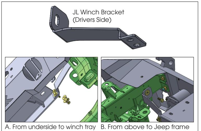
9. Now install passenger side JL winch bracket. The bracket mounts to the winch tray with two M8 bolts with flat, lock washers and nuts. Next mount to the Jeep frame with M10 bolt and flat washer.
