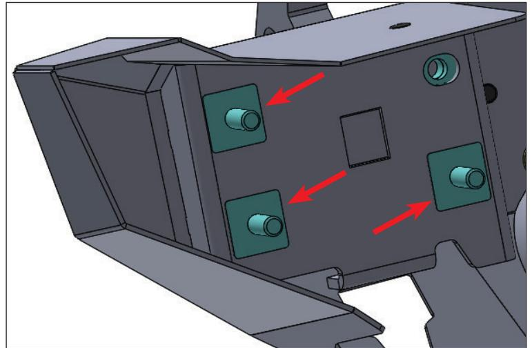
5. Now lift and place the bumper to the Jeep frame rails. The studs slide through the holes in the frame holes. It's best to have an assistant to lift and hold the bumper in place.
