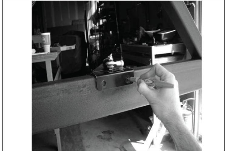
5. Use the supplied M10 Self-Tapping bolts to tap threads into the holes in the horizontal beam.
