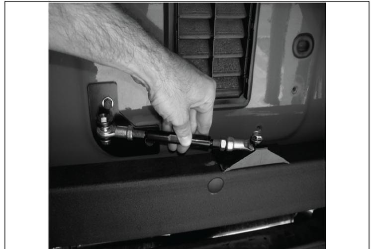
3. Mark the location of the outer edge of the Tire Carrier Bracket on the horizontal beam of the tire carrier with tape.
