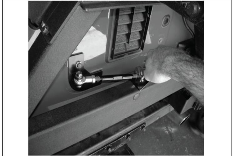
8. This product will work differently with different tire carriers. Always open or close the tailgate first then release or attach the tire carrier latch. The latching mechanism of some tire carriers may interfere with the closing of the tailgate. In this case, it may be necessary to close the tailgate while holding the tire carrier latch in the open to avoid interference.
