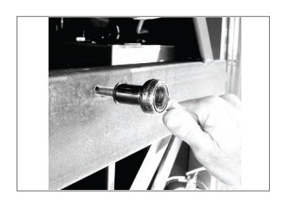
6. Install the Tire Carrier Bracket to the horizontal beam of A-frame tire carrier using the M10 Self-Tapping Bolts.
