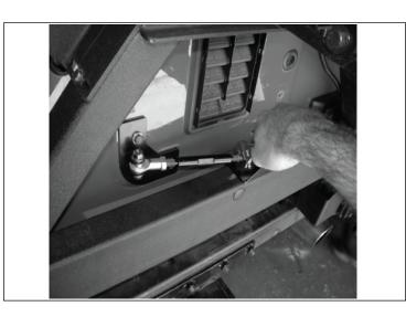
8. This product will work differently with different tire carriers. Always open or close the tailgate first then release or attach the tire carrier latch. The latching mechanism of some tire carriers may interfere with the closing of the tailgate. In this case, it may be necessary to close the tailgate while holding the tire carrier latch in the open to avoid interference.
