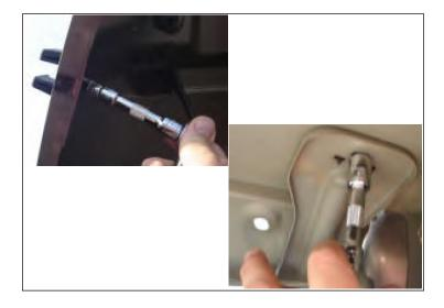
2. Install upper lock assemble to vehicle. Install (2) stainless washer, and (2) Nylock nuts to each assemble. Tighten bolts. Make sure the lock face is pointed towards the rear of the hood. Insert Lock Post into the lock assemble heads as seen in and turn lock to hold in place. Lower hood to see if they align with center mounting hole in the fender. If they do not align correctly additional adjustments may be needed to hood or fenders.
