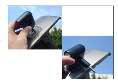
3. Remove plastic protective cover from Lock Post stainless steal cover plate like shown below. Place Lock Post rubber gasket and cover plate on fender and align the center mounting hole. Remove Lock Post from lock assemble and unscrew top cap to expose Allen head bolt. Insert into cover plate as seen in.
