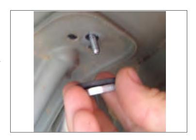
5. Additional washers are supplied to raise the Lock Post if needed. Install washers as needed for proper fitment.
